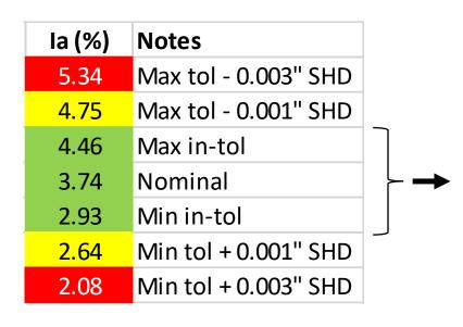
Within nominal Cx process tolerances, the predicted LIF  $\sim 2.5 ... 31.0$  using a = 0.300" as a reference point:
