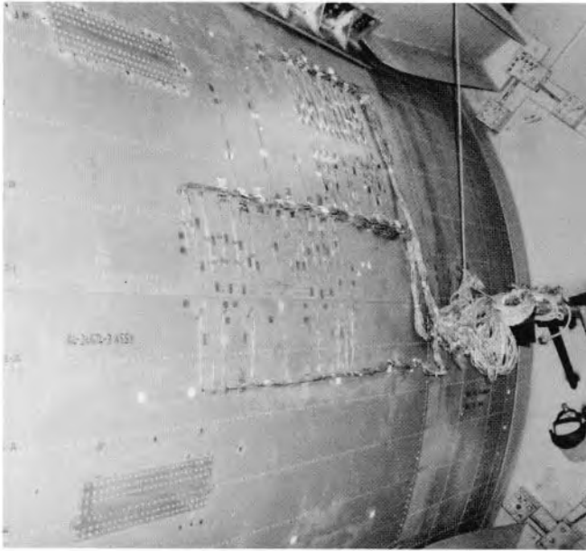
Figure 8. Typical Fuselage Pressure Test Panel
