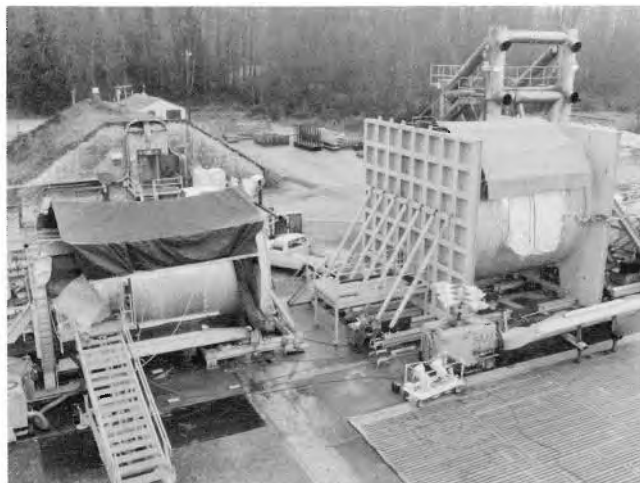
Figure 7. Fuselage Pressure Test Fixtures
