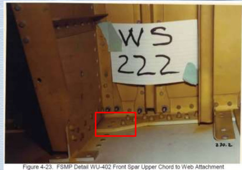
Figure 4-23. FSMP Detail WU-402 Front Spar Upper Chord to Web Attachment
