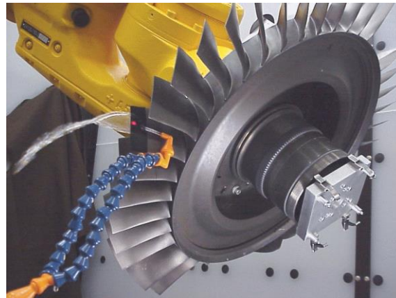
F119 engine IBR being laser shock peened. Source: http://www.lsptechnologies.com/production-uses/
