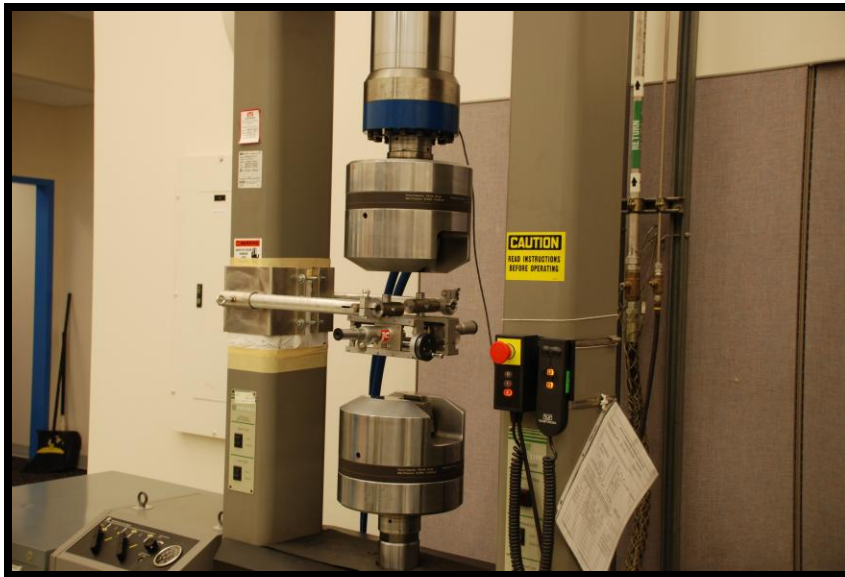
Fig. 3 MTS grip set-up with traveling microscopes.
