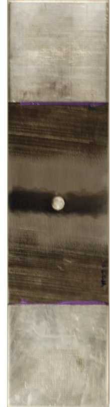
Fig. 2 Final specimen preparation for cold expanded specimens.
