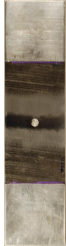
Fig. 2 Final specimen preparation for cold expanded specimens.
